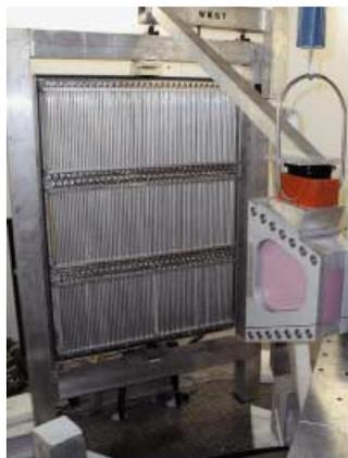
Fig. 4. Radial collimator supported in front of detector
