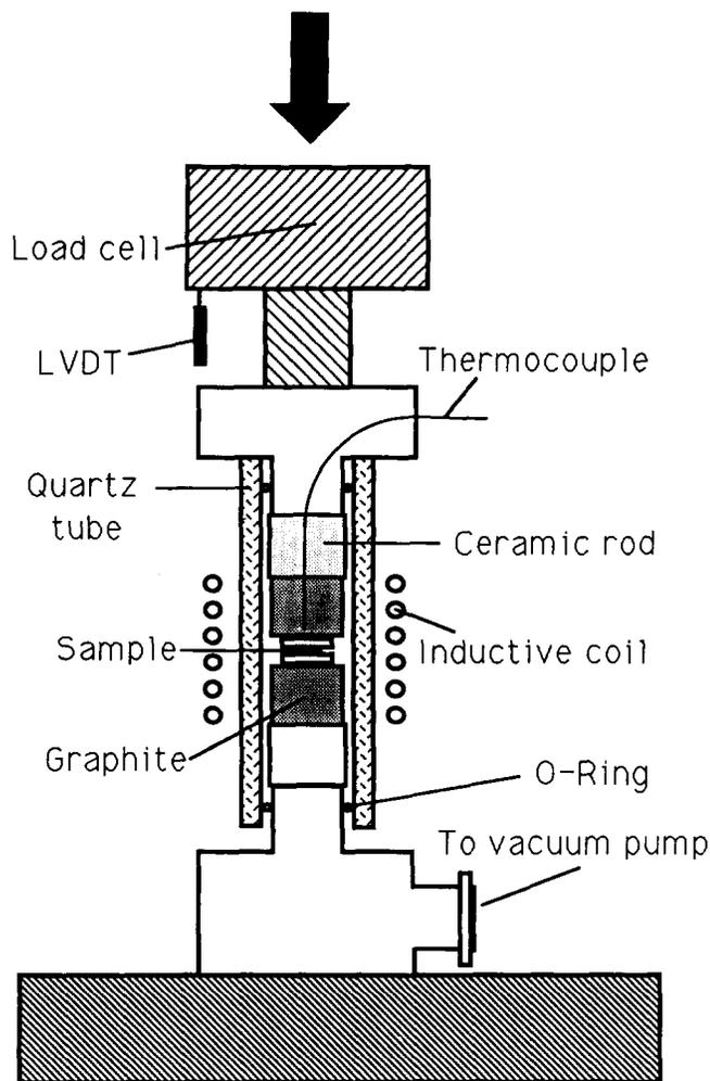
Fig. 2 Schematic of hot-pressing apparatus
