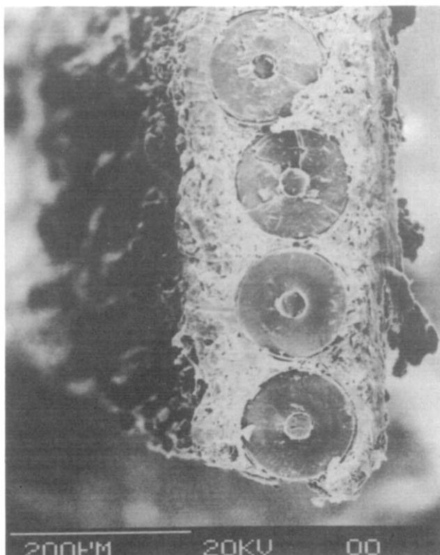
Fig. 1 Scanning electron micrograph of as-received fibre-rich SCS-6™ monotape
