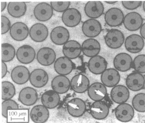
Fig. 4 Optical micrograph of a compacted sample showing a stack of touching fibres forming an arch shielding a matrix region with pores (arrows), while the surrounding unshielded matrix is virtually pore-free (SCS-6™ fibre, 900°C, 40 MPa). The external load was applied in the vertical direction of the micrograph
