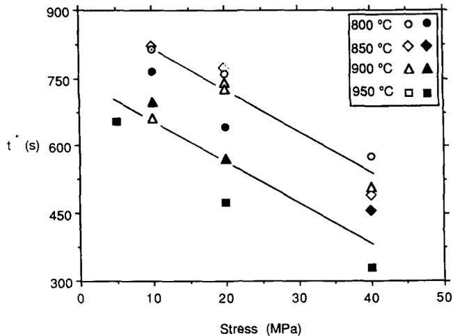
Fig. 3 Time  $t^*$  as a function of applied stress and temperature for matrix-rich specimens (open symbols) and fibre-rich specimens (filled symbols) of Sigma™ fibre-reinforced titanium monotapes
