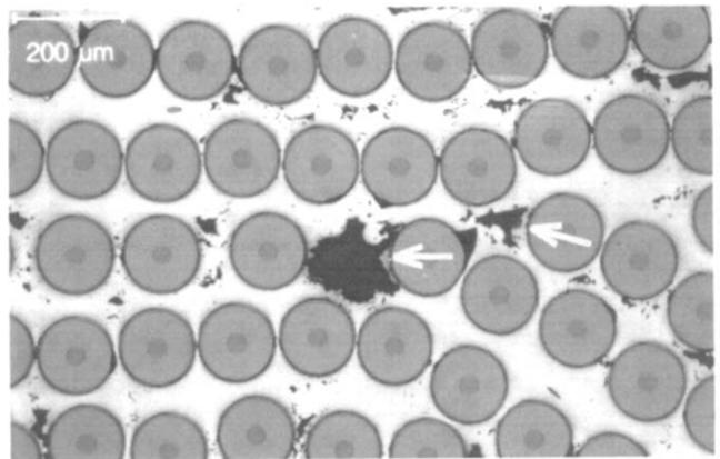
Fig. 5 Optical micrograph showing porosity (arrow) resulting from narrow monotapes sandwiched between broader monotapes (SCS-6™ fibre, 850°C, 20 MPa)
