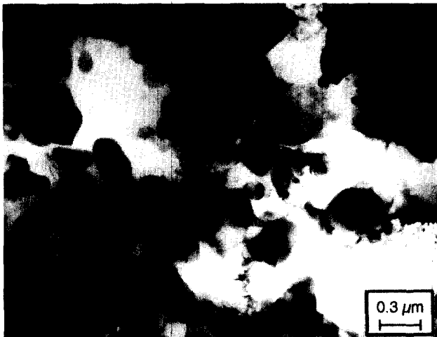
Fig. 3. Transmission electron micrograph of ODS-Al extruded at 550 °C showing improved particle distribution.
