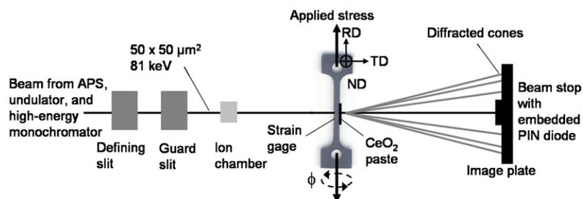
Fig. 1. Schematic of experimental diffraction setup, showing photograph of a UHCS tensile sample with rolling (RD), transverse (TD) and normal (ND, out of the page) directions indicated.
