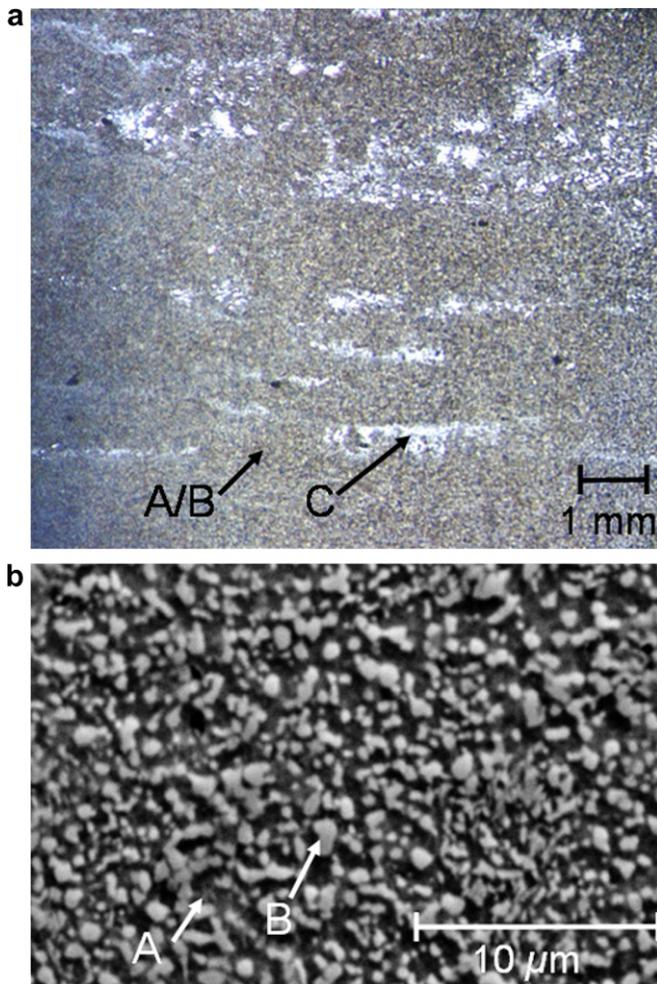
Fig. 3. (a) Optical micrograph of the UHCS sample etched with 2% Nital showing a region of  $\alpha$ -Fe matrix and  $\text{Fe}_3\text{C}$  spheroids (A/B) and large striations of proeutectoid  $\text{Fe}_3\text{C}$  (C). (b) Scanning electron micrograph in secondary electron mode of a UHCS sample etched with 2% Nital with  $\alpha$ -Fe matrix (A) and  $\text{Fe}_3\text{C}$  spheroids (B) indicated.
