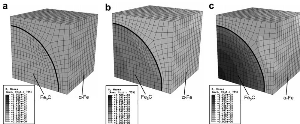
Fig. 10. Finite-element model showing the von Mises stress distribution (a) before Lüders band propagation at 700 MPa; (b) after Lüders band propagation at 700 MPa, and (c) at a maximum load of 1100 MPa. One-eighth of the  $\text{Fe}_3\text{C}$  sphere and the surrounding  $\alpha$ -Fe matrix are shown.
