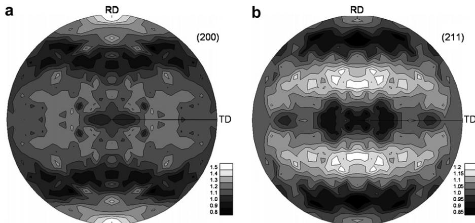
Fig. 4. Pole figures with no applied stress for the (a) (200) and (b) (211)  $\alpha$ -Fe reflections. Scale shows MRD values.
