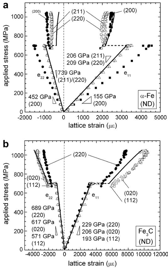
Fig. 9. Applied stress vs. lattice strain for (a) the  $\alpha$ -Fe (200), (220) and (211) reflections, and (b) the  $\text{Fe}_3\text{C}$  (020), (220) and (112) reflections, for beams parallel to the ND. The values of the slopes represent best fit of the experimental data. Average elastic strains from finite-element modeling are shown as solid lines (dashed lines in the Lüders region are shown for continuity).
