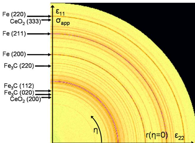
Fig. 2. Representative X-ray diffraction pattern (quarter of image plate) of the UHCS sample. All of the diffraction rings were identified. For clarity, only some of the rings belonging to  $\text{CeO}_2$ ,  $\alpha$ -Fe, and  $\text{Fe}_3\text{C}$  phases are indicated here. Darker pixels indicate higher diffracted intensity.
