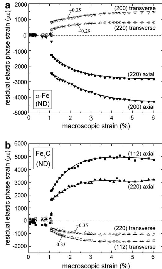
Fig. 11. Residual elastic phase strains in (a)  $\alpha\text{-Fe}$  for (200) and (220) reflections and (b)  $\text{Fe}_3\text{C}$  for (220) and (112) reflections vs. macroscopic steel strain. The solid lines for the axial strains are best-fit curves through the data points. The dotted lines for the transverse strains are produced by multiplying the solid lines by a factor indicated next to the lines.
