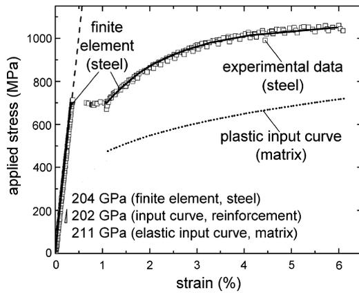
Fig. 5. Macroscopic stress–strain curve for UHCS tensile sample showing experimental data (open squares),  $\alpha$ -Fe and  $\text{Fe}_3\text{C}$  reinforcement elastic input curve (dashed line),  $\alpha$ -Fe matrix plastic input curve (dotted line), and steel curve calculated from finite-element model (solid line). The model does not capture the Lüders band propagation between the elastic and plastic ranges.
