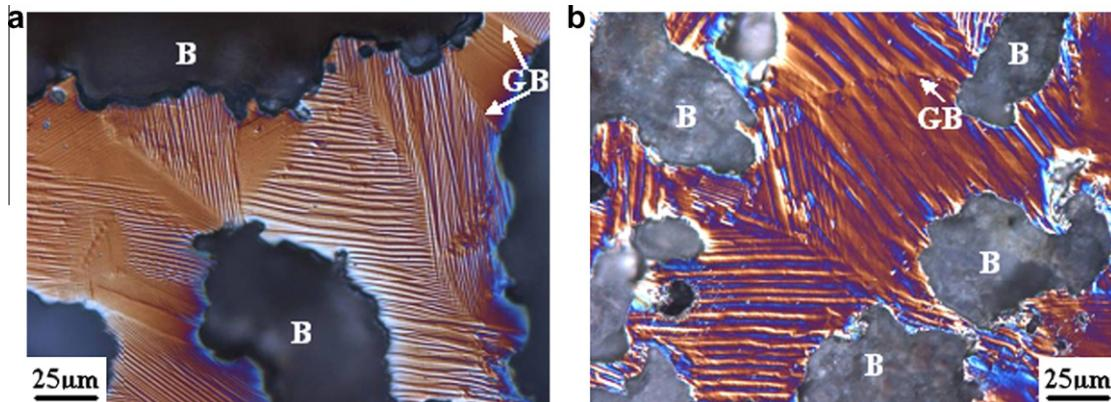
Fig. 5. Optical micrographs of polished cross-sections of dual-pore foam in area with small pores (B) imaged with polarized light. (a) As-cast state, with fine twins, many of which do not span the width of the struts. Bamboo grain exists on slender struts; (b) annealed state, with coarser twins spanning the whole width of the nodes and struts. A grain boundary (GB) at a node is also visible.
