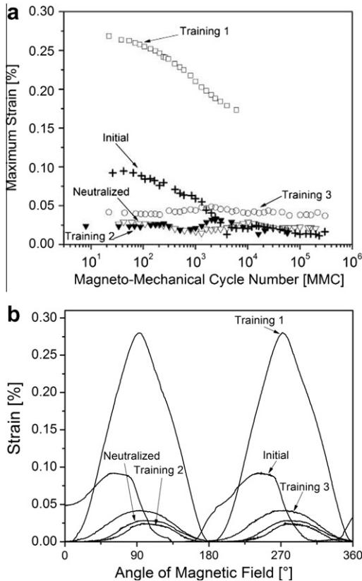
Fig. 9. MFIS of dual-pore foam with 66.8% porosity. (a) MFIS vs. MMC for five different states: as-annealed, first training, neutralized, second training and third training; (b) MFIS vs. magnetic field orientation for the same five states.
