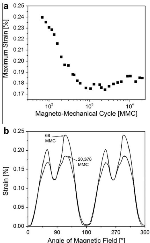
Fig. 8. MFIS of single-pore foam with 56.6% porosity. (a) MFIS vs. MMC; (b) MFIS vs. magnetic field orientation for 68 and 20,378 MMC.
