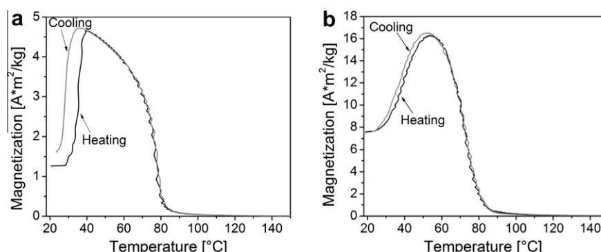
Fig. 7. Magnetization–temperature curve of Ni–Mn–Ga foam measured with a VSM. (a) Foam of the annealed state with single pores in a 0.0326 T magnetic field; (b) foam of the annealed state with dual pores in a 0.028 T magnetic field.
