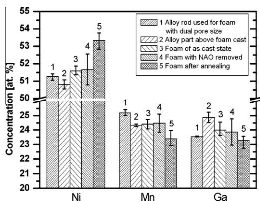
Fig. 6. Compositional evolution of dual-pore foam during processing.
