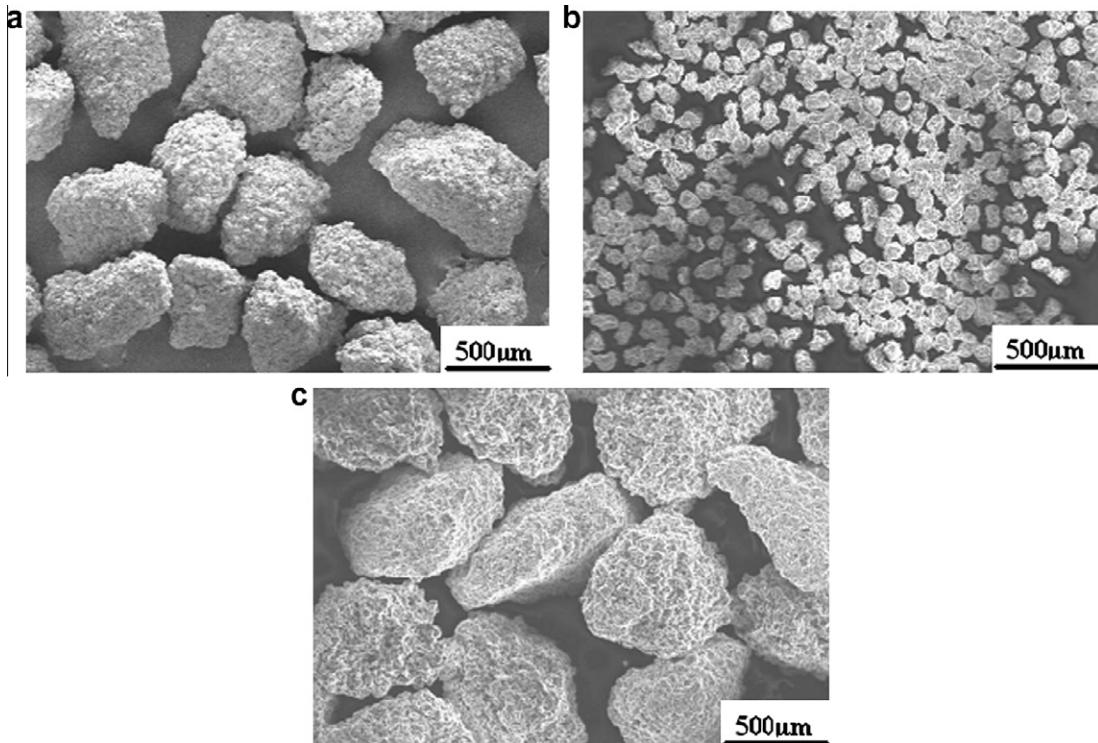
Fig. 1. SEM micrographs of  $\text{NaAlO}_2$  powders with different sizes used as a space holder to prepare the Ni–Mn–Ga foams: (a) 355–500  $\mu\text{m}$  powders, (b) 75–90  $\mu\text{m}$  powders, (c) 500–600  $\mu\text{m}$  powders.
