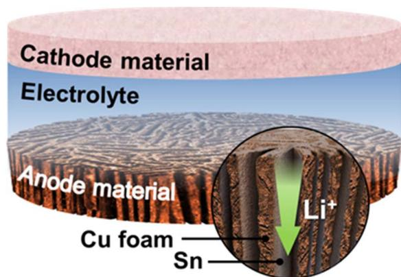
**Fig. 1.** Schematic of a lithium-ion battery design containing a freeze-cast Cu foam coated with Sn, with high permeability and open space to accommodate Sn (de)lithiation volume changes, which may be used as both the anode and current collector to enhance efficiency and cycling resistance during the (dis)charging process.
