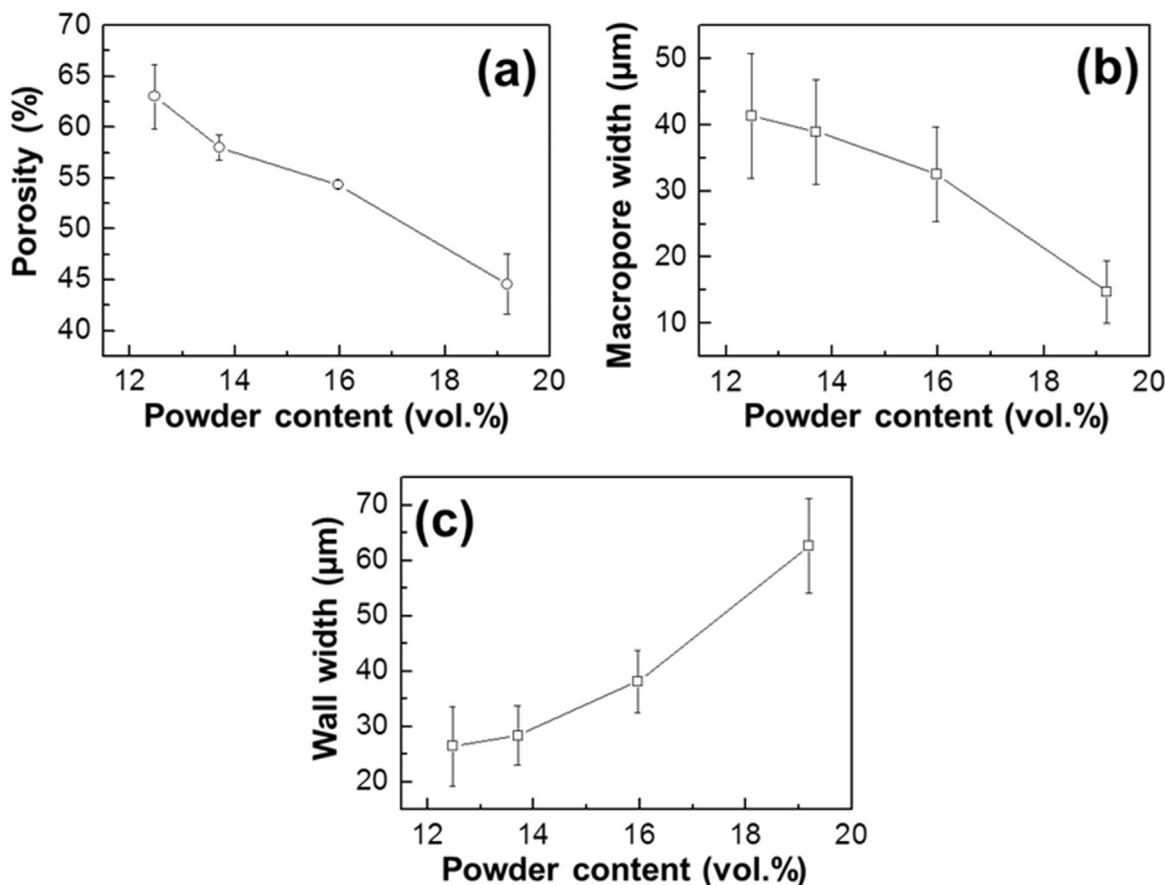
Fig. 9. Plots of (a) porosity, (b) macropore width, and (c) wall width against oxide powder content in slurry at constant casting temperature of  $-15\text{ }^{\circ}\text{C}$  (foams V13, V14, V16, and V19).
