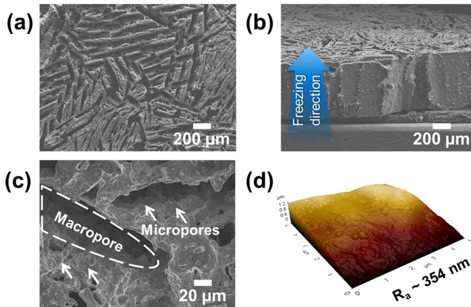
**Fig. 4.** SEM and AFM images of Cu foam V14 with a hierarchical pore structure: (a, b) lamellar macropores created by the ice dendrites during freezing, (c) micropores on the Cu walls, and (d) AFM image of the as-cast top morphology of the freeze-cast Cu foam with a mean surface roughness ( $R_a$ ) ~350 nm.
