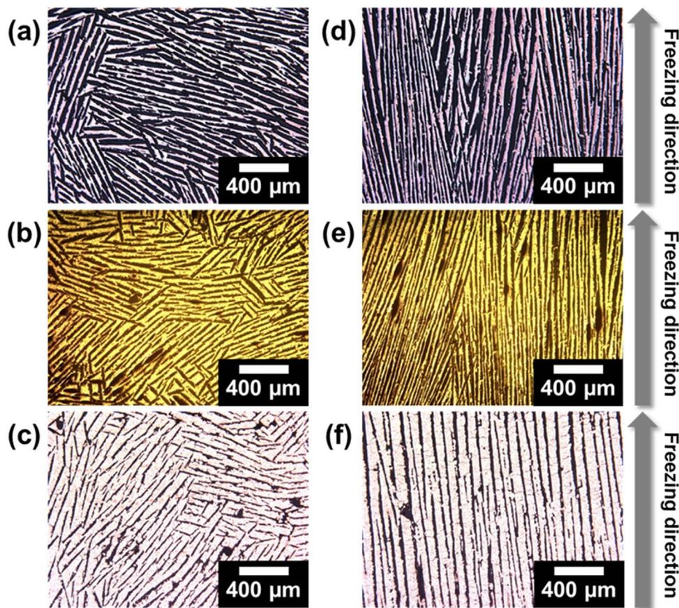
**Fig. 8.** Optical micrographs of (a–c) radial and (d–f) longitudinal cross-sections of center region of Cu foams solidified at  $-15^{\circ}\text{C}$  from slurries with increasing oxide powder fractions: (a, d) 12.5 vol% (foam V13), (b, e) 16.0 vol% (foam V16), and (c, f) 19.2 vol% (foam V19).
