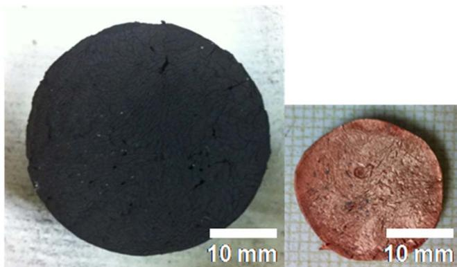
**Fig. 2.** Photographs of freeze-cast foam V13 after freeze drying (left) and after subsequent reduction and sintering (right), illustrating the color change from black CuO to light red Cu and considerable volume shrinkage without cracking or warping. (For interpretation of the references to color in this figure legend, the reader is referred to the web version of this article.)
