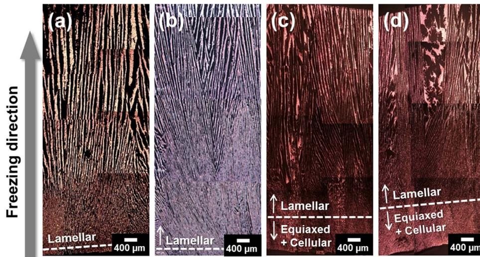
Fig. 6. Optical micrographs of longitudinal cross-sections of Cu foams created from slurries with 12.5 vol% oxide particles solidified at decreasing casting temperatures: (a) -10 (T10), (b) -15 (T15), (c) -20 (T20), and (d) -30 (T30) °C. The transition between a cellular region near mold bottom and a lamellar pore region is marked with a dotted line.
