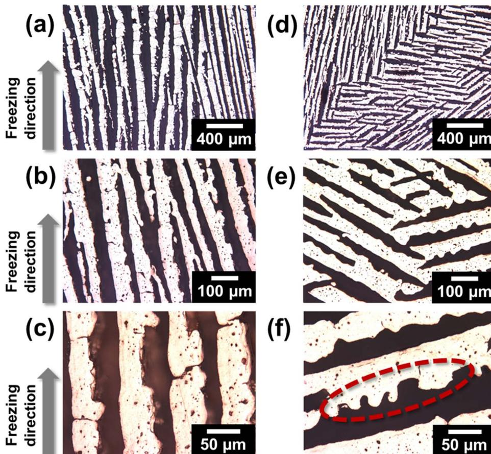
**Fig. 3.** Optical micrographs at various magnifications of Cu foam V13 showing (a, b, c) the lamellar macropore structure and (d, e, f) the morphology of the macropores and Cu walls, containing microporosity at their surface (circle) and, to a modest extent, within their volumes.
