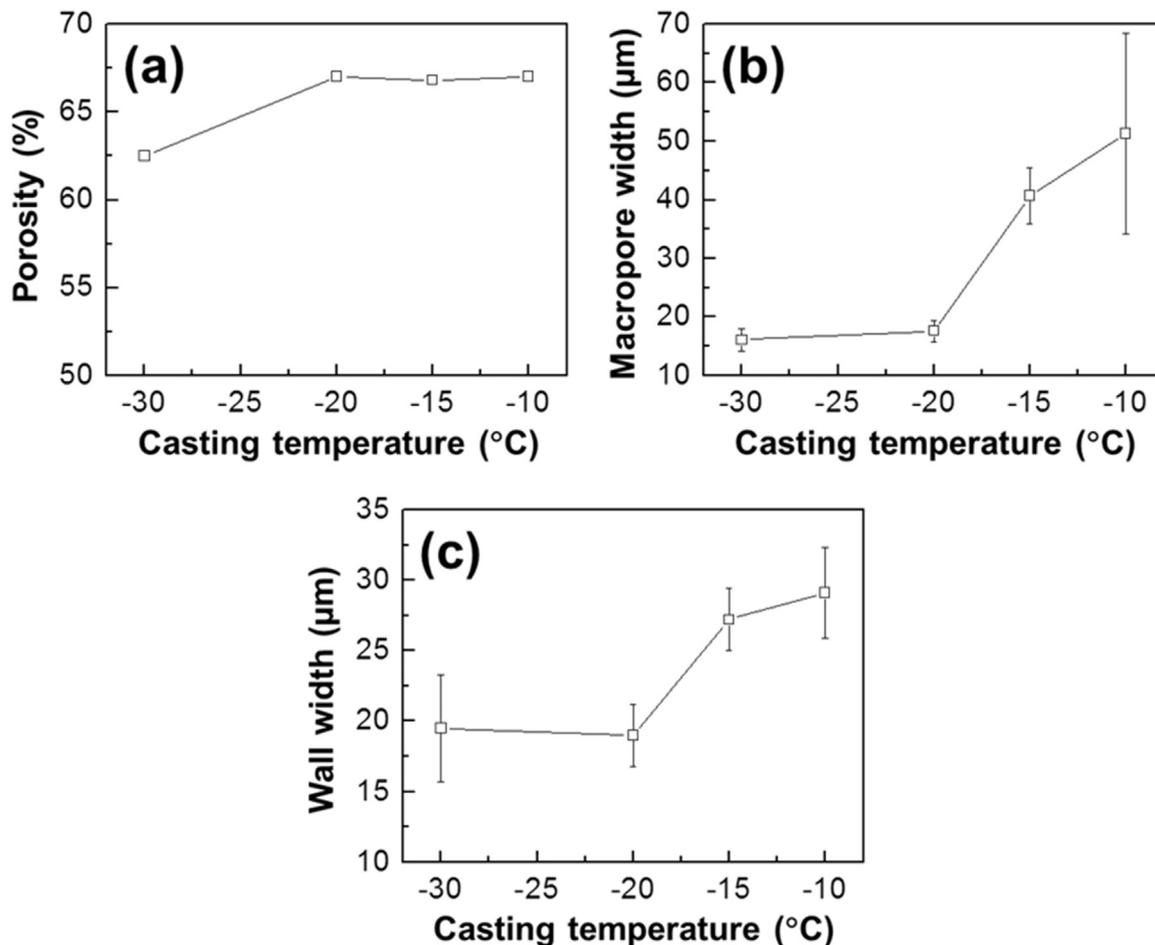
Fig. 7. Plots of (a) porosity, (b) macropore width, and (c) wall width against slurry casting temperature at constant slurry volume fraction of 12.5% (foams T10, T15, T20, and T30).
