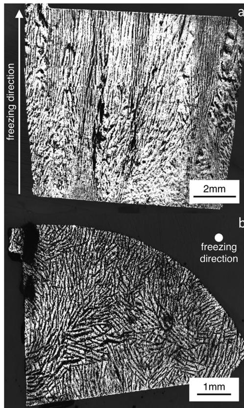
**Fig. 1.** Optical micrograph of iron foam reduced and sintered from 20 vol.%  $Fe_2O_3$  slurry. Cross-sections are (a) longitudinal, showing short-range lamellar channel structure consistent with conventional unidirectional freeze-casting [3] separated by Fe walls, and (b) radial, showing lamellar channels parallel to each other within colonies of consistent size.
