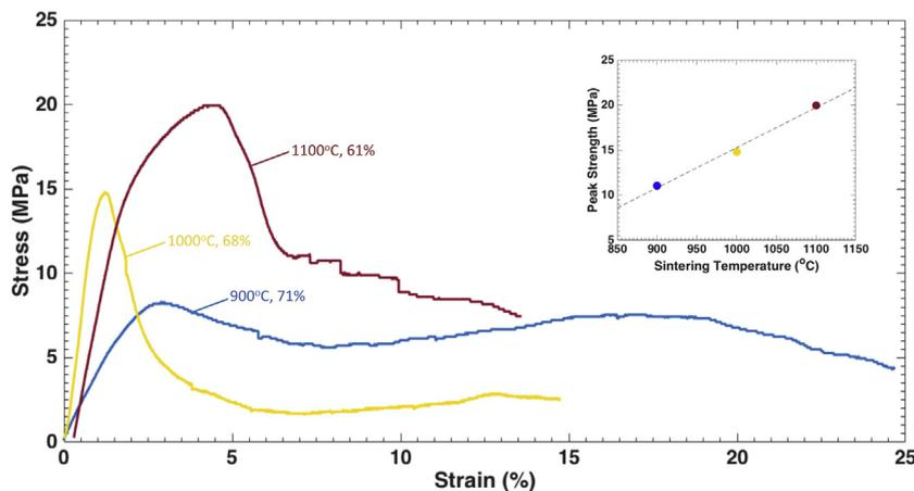
**Fig. 4.** Compressive stress-strain curves for foams freeze-cast from 18.5 vol.%  $\text{Fe}_2\text{O}_3$  slurry, sintered at various temperatures and with various porosities. Inset: Yield strength of foams as a function of sintering temperature. There are no error bars because we were only able to complete one compression test for each sintering temperature.
