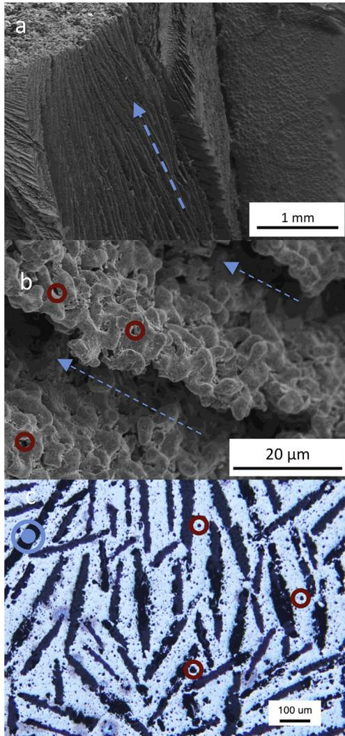
**Fig. 3.** Arrows indicate freezing direction and red circles show micropores within channel walls. (a) SEM micrograph showing wall microstructure of Fe foam reduced and sintered from a 20 vol.%  $\text{Fe}_2\text{O}_3$  slurry. (b) High-magnification SEM micrograph of channel walls with extensive surface porosity. (c) Optical micrograph of radial cross-section showing micropores within channel walls.
