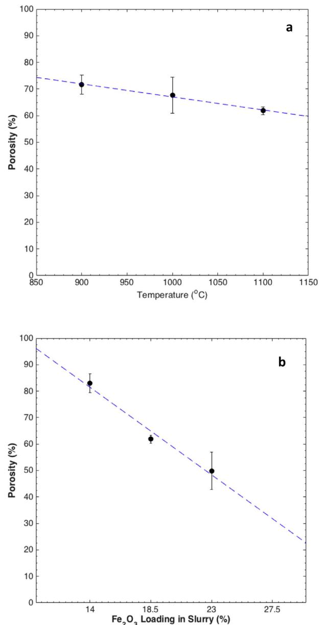
**Fig. 2.** Effect on foam porosity of (a) sintering temperature at constant  $Fe_2O_3$  slurry fraction of 18.5 vol.%, and (b)  $Fe_2O_3$  slurry fraction at constant sintering temperature of 1100 °C.
