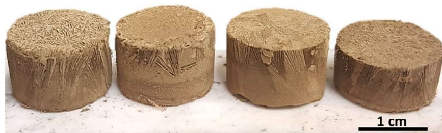
Figure 1. Ice-templated Si foam after sintering displaying lamellar porosity. Solidification temperature varied from left to right: –10, –15, –20, and –25 °C. The same volume of suspension was used to solidify all samples.
